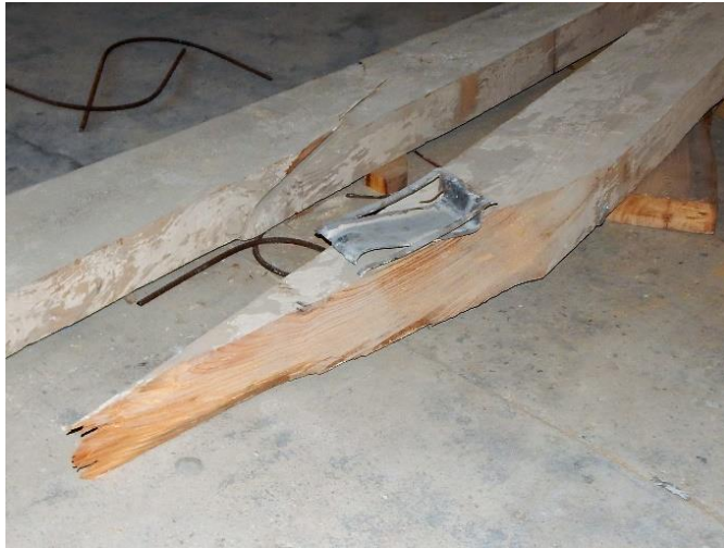
Figure 27 Failure due to excessive slope of grain
