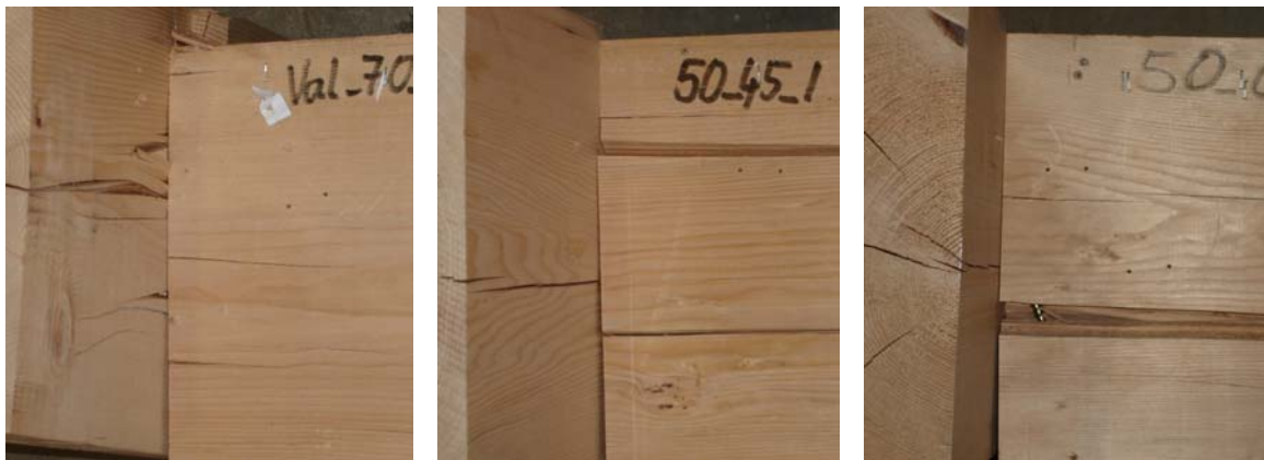
Figure 10-6: Typical failure modes of reinforced RDC: 90^\circ (left), 55^\circ (centre), crossed (right)
