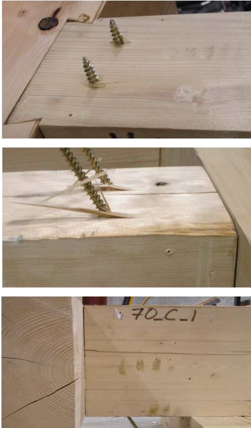
Figure A-12: Reinforced test specimens: 90° (top), 55° (middle), cross (bottom)
