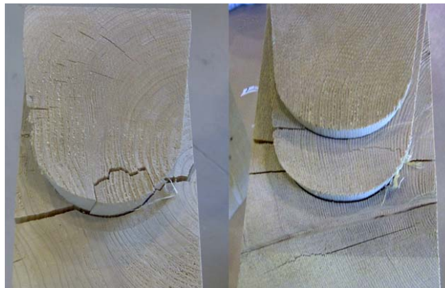
Figure 2-7: Typical failure of RDC (left) and DRDC (right)
