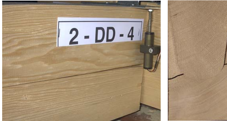
Figure 8-2: Typical failure of RDC in shear test
