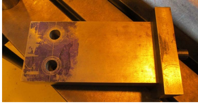
Figure 1. Steel Tenon Used for Mortise Member Testing
