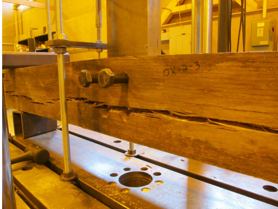
Figure 7. Split Failure Extending Through Previously Tested Bolt Holes
