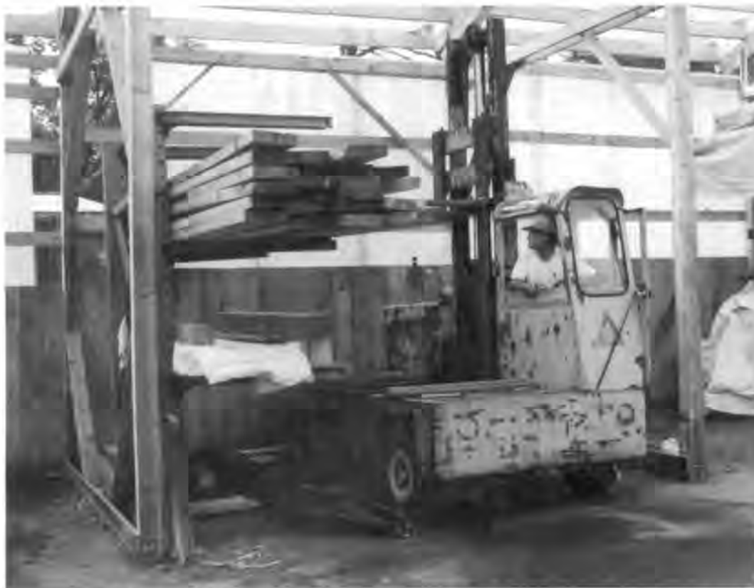
British-made Allis-Chalmers forklifts work to the side of the chassis and can sneak into confined bays. One has a capacity of 11,000 pounds.
