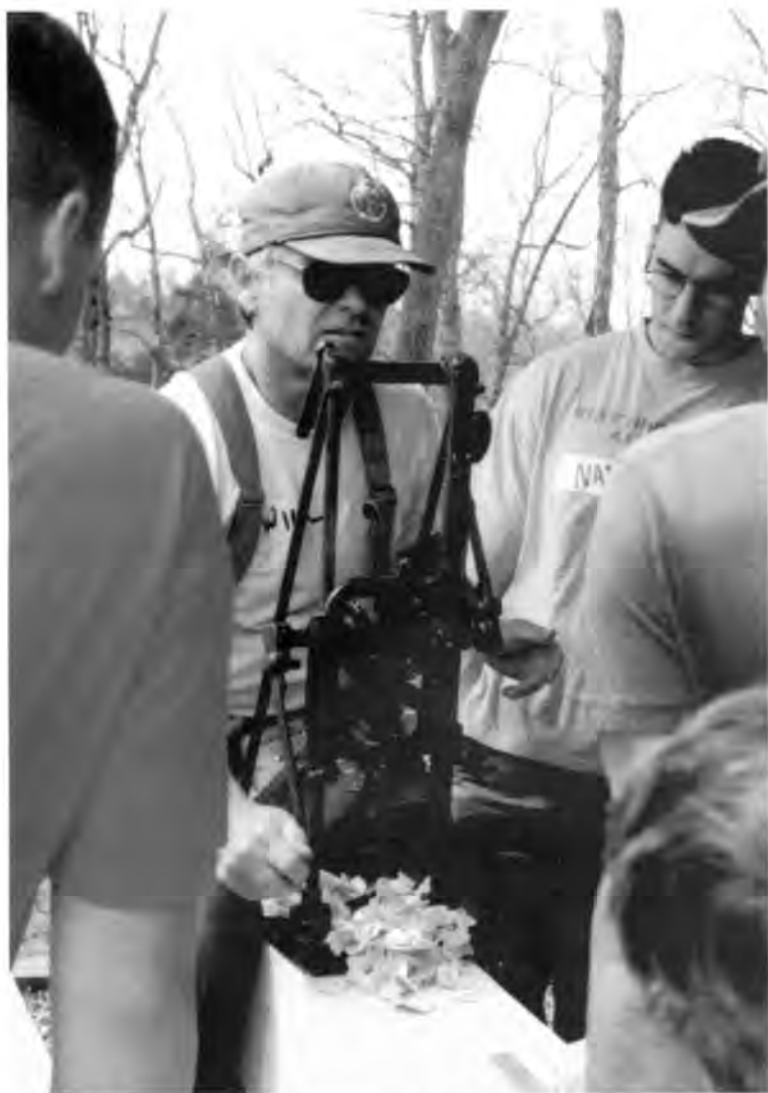
Will Beemer incognito demoing the Millers Falls boring machine.
