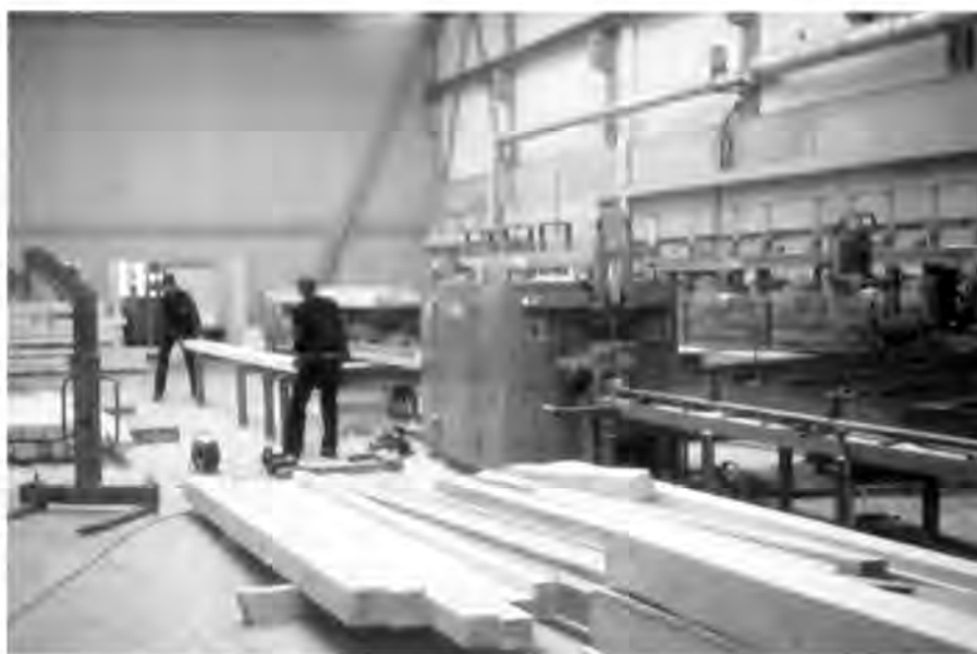
The Hundegger system produces nearly finished pieces from blank timbers. Like the shoemaker's elves, it can also work while the master is away.
