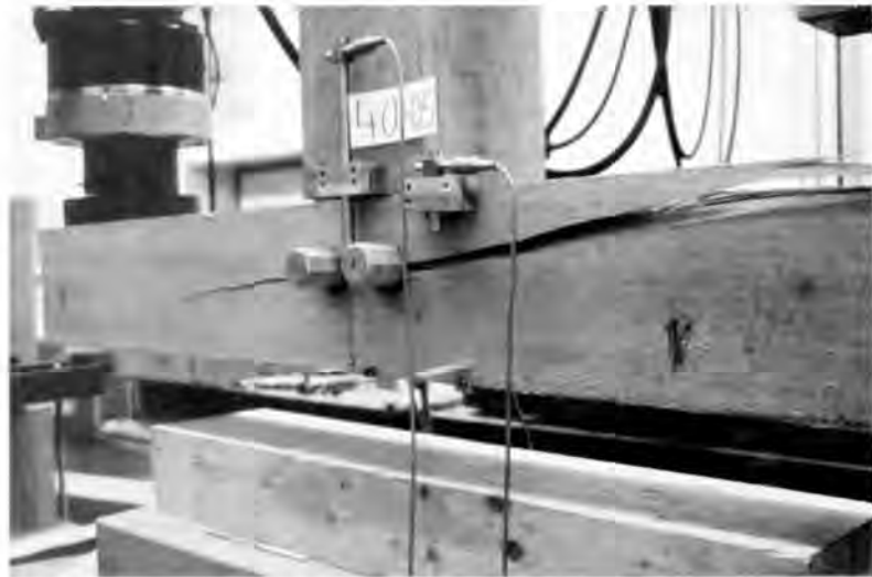
Mortise housing break, 90° connection.
