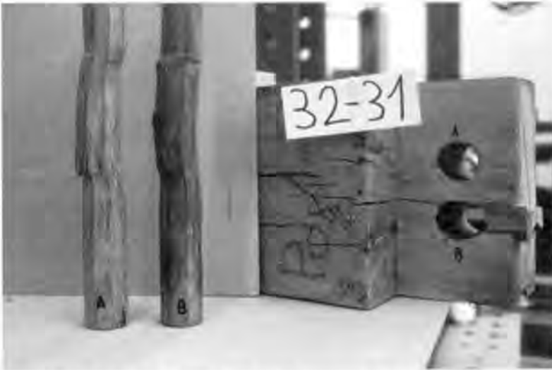
Peg break (left) and shear break in the tenon, 90° connection.
