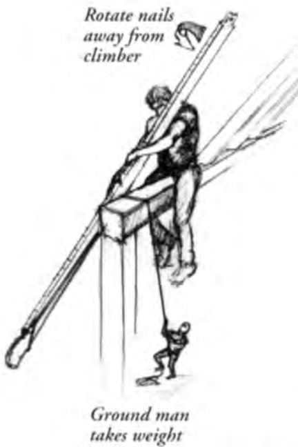
FIGURE 2 REMOVING RAFTERS
