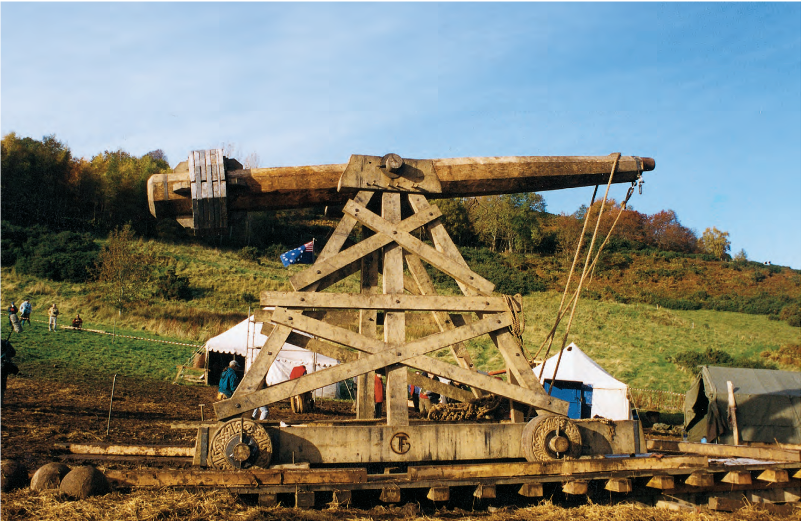
Figurado, the fixed-counterweight machine, complete, mounted on its track.
