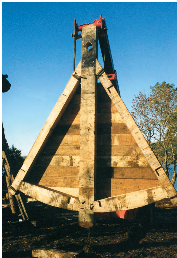
Above, the counterweight basket before mounting to the rest of the trébuchet at right.
