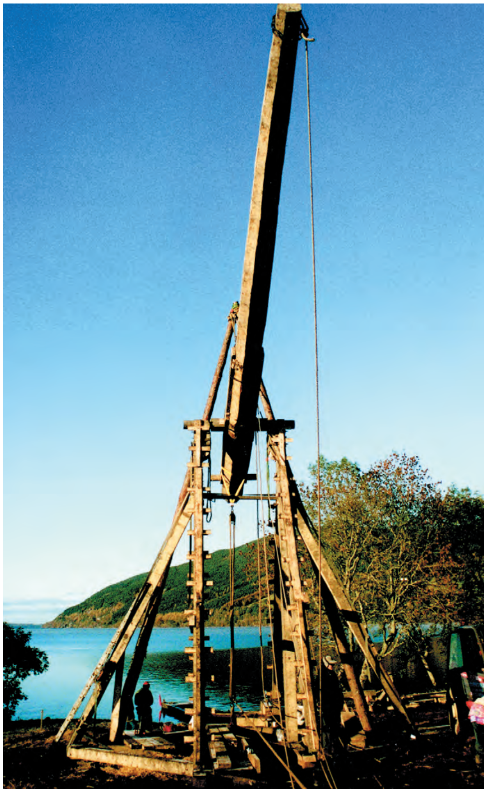
At rest, the hinged-counterweight machine stands nearly 54 ft. high.
