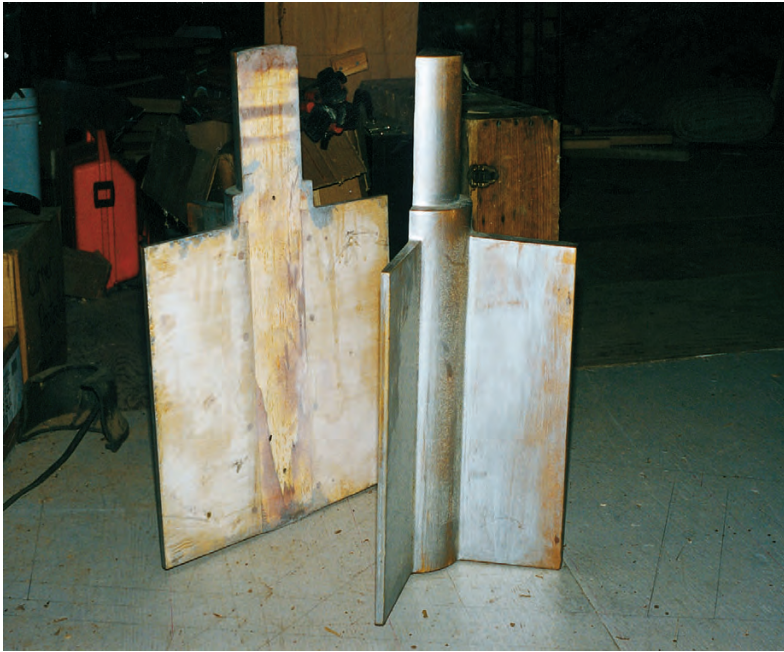
Above, split pattern for casting iron gudgeon shown below installed in shaft log for 1991 water wheel in Lake Buena Vista, Florida. At right, Rondout's Wayne Ford with wooden gears for the same job.
