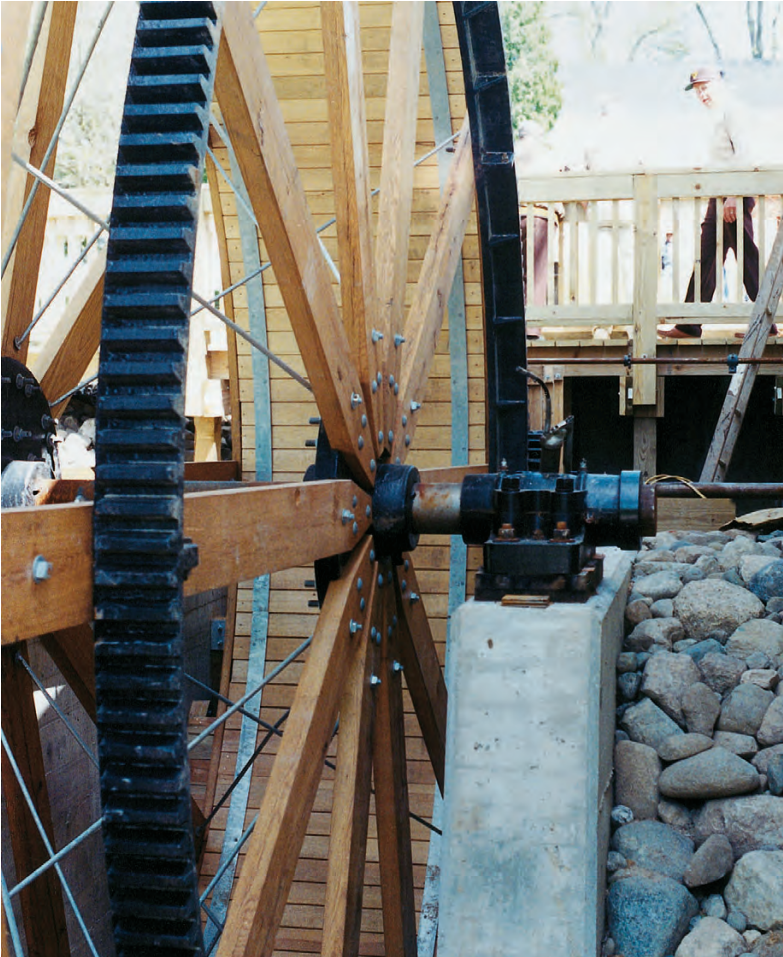
Below left and below, 20-ft. low-breast water wheel in Ray Township, Michigan, with wooden buckets and arms, cast iron hubs and a 16-ft. cast iron segment gear and pinion.
