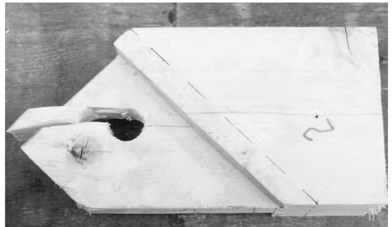
FIGURE 5. TENON RELISH FAILURE (PORT ORFORD CEDAR).
