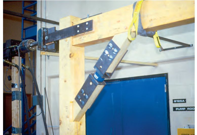
FIGURE 9. PORT ORFORD CEDAR KNEE BRACE LOAD CELL.
