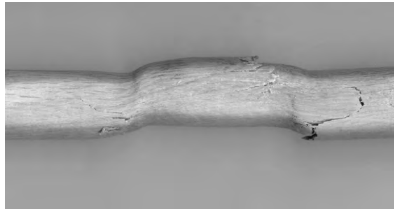
FIGURE 4. PEG COMBINED SHEAR AND FLEXURE FAILURE.
