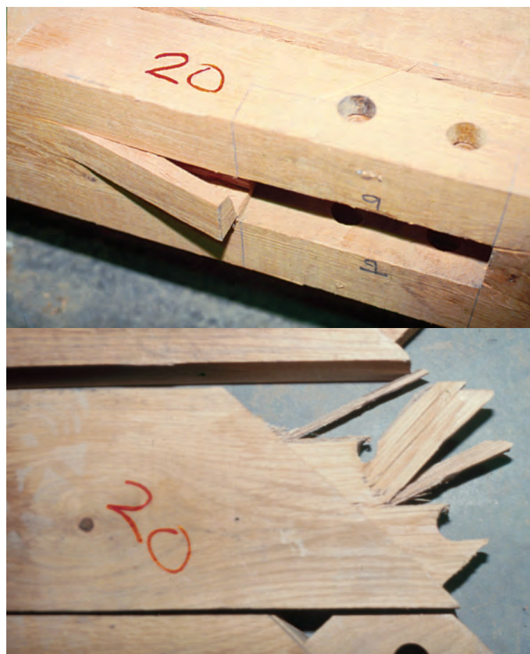
FIGURE 3B. COMPLETE DESTRUCTION OF BRACE TENON AND DAMAGE TO MORTISE AT JOINT 20 (OAK FRAME).
