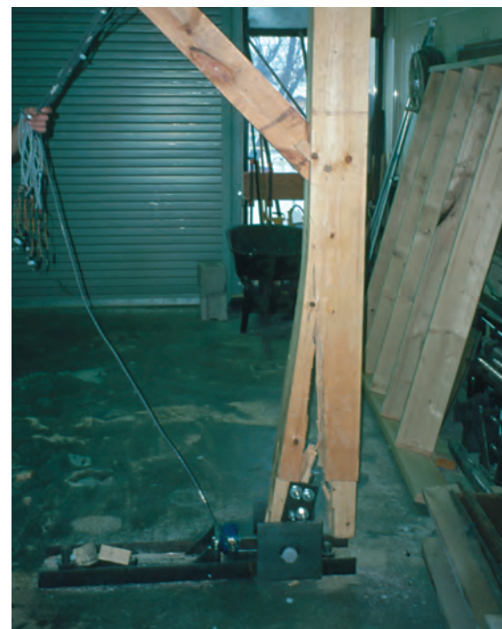
FIGURE 3. WHITE PINE POST FAILURE AT TEST FIXTURE (REACTION CONNECTION).
