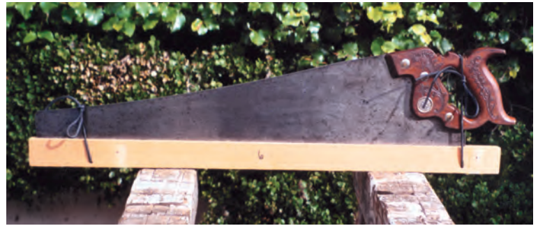
To protect a sharp handsaw, make a guard of softwood by slotting a 3/4-in.-deep groove the length of a 1x3. Thread two rawhide strings through holes drilled in the bottom of the guard to tie it on.
