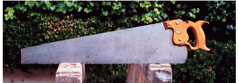
Disston D-7, ca. 1895, 5 1/2-pt. rip saw with quartered beech handle, an old and beautiful pattern, but often too small for all four fingers.
