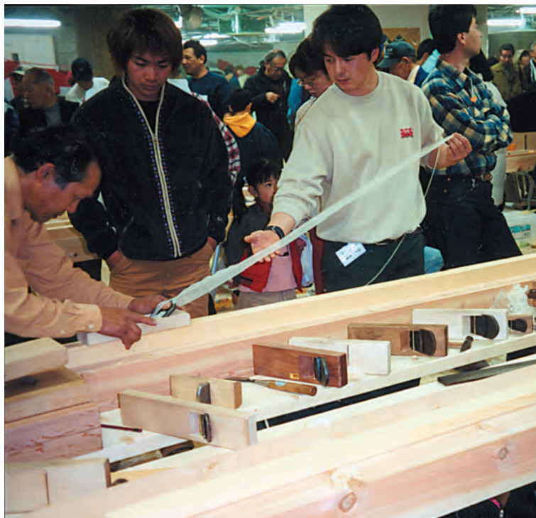
Kezurou-Kai, a group devoted to woodworking skills, above all hand planing, gathers semi-annually for a best-shaving competition and exposition of tools and techniques. Shaving at right mikes at 17 microns.
