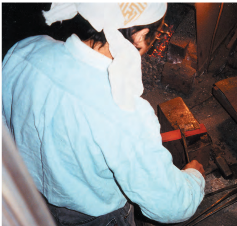
Funahiro-san prepares to forge-weld the harder steel that will form the working edge of a chisel to the milder steel that will make up the body.
