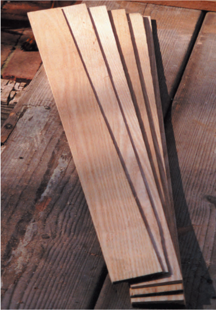
Eighth-in. ash strips sawn out of 8/4 stock 2½ in. wide and set on edge.
