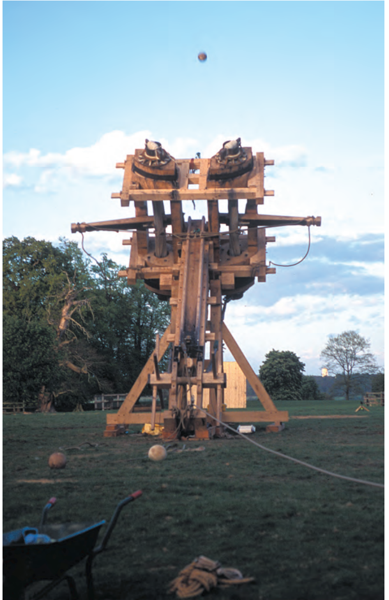
The missile placed, and nearly everyone (including the photographer) having withdrawn to a safe distance, the trigger has been pulled remotely and the missile has launched, guided by the slider. The bow arms travel through a remarkably short arc to accomplish their work.
