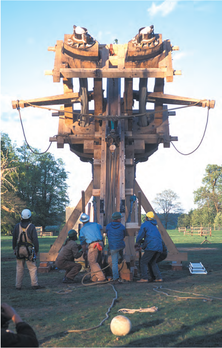
The slider, the long channel-shaped box at the center of the machine, has been winched up and the bowstring attached, and now the crew has begun the laborious job of winching down against the vast resistance of the pretensioned skeins. Hand-carved stone ammo in the foreground.
