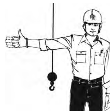
Boom up, cable down (flex fingers).
