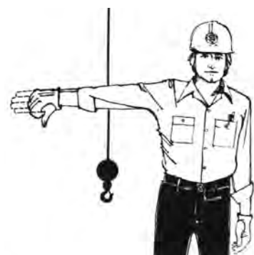
Boom down, cable up (flex fingers).
