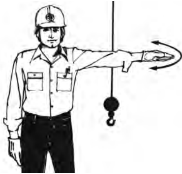
Stop. Palm down, move hand laterally.
