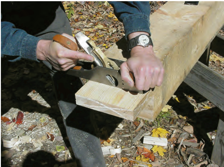
Bench rabbet plane will work the cheek right up to the shoulder (and will trim the shoulder square if necessary).
