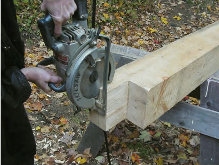
The dive or drop cut is an efficient method to remove waste in one step.
