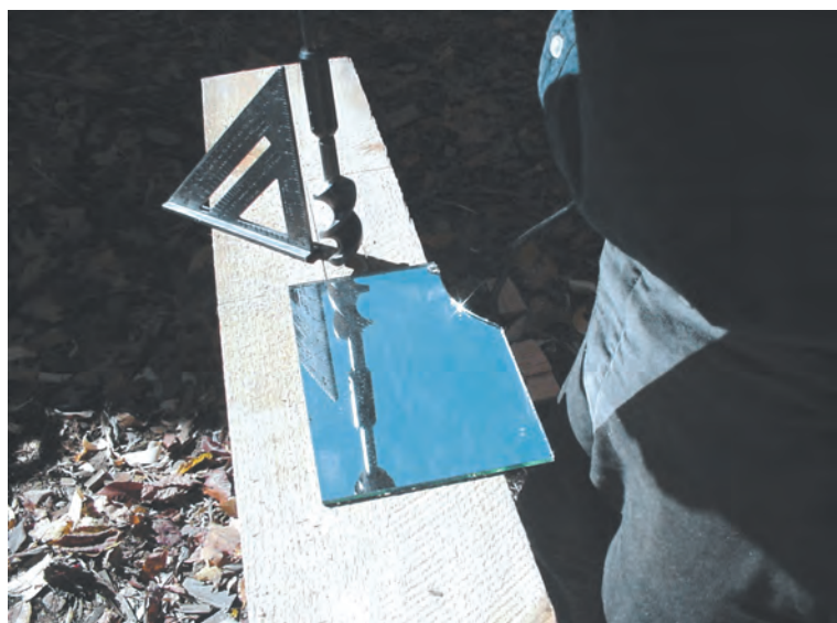
Drilling out for a mortise using aids to keep square to good top surface.
