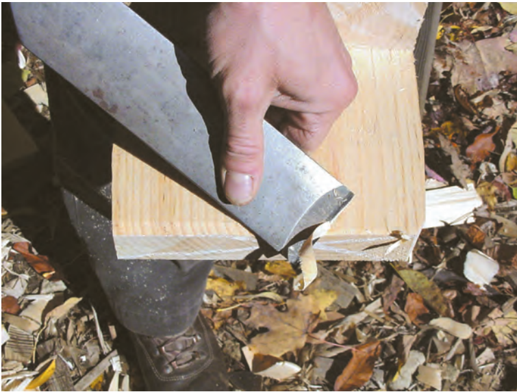
Chamfering the tenon arris for easy assembly.
