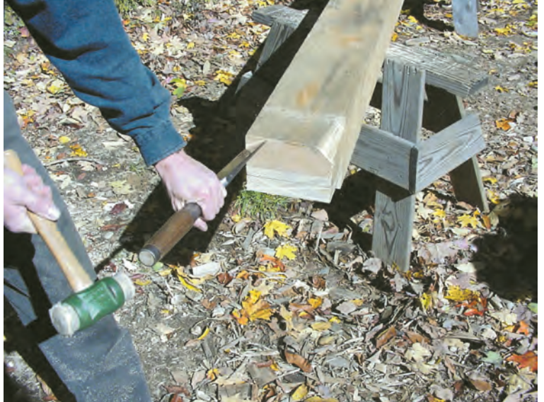
In straight grain, most waste can be quickly removed with a chisel.
