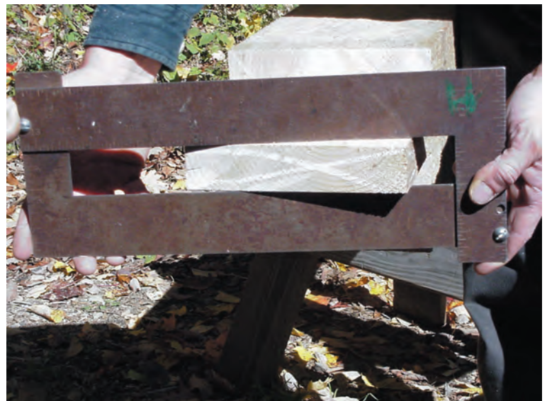
Tenon thickness checker made from cut-down framing squares and adjustable for 1½-in. and 2-in. tenons. Temporary checker can be made from full-size squares clamped by stair gauge fixtures.
