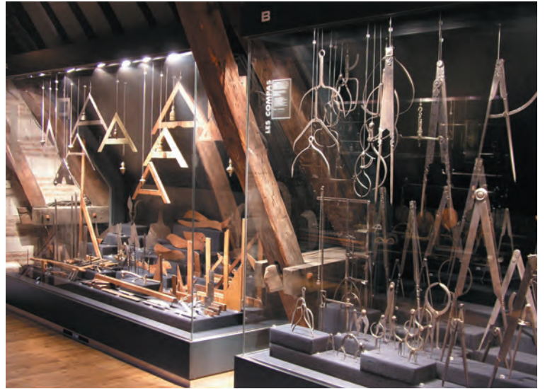
Display of measuring tools at the Maison de l'outil in Troyes. Notice the jambe de force, or leg of strength, rising between the showcases and stoutly connected to the principal rafter by a triple-tenoned link.
