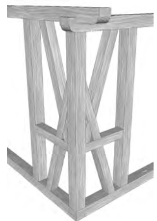
Fig. 4. K-Runes brace pattern at a corner post.
