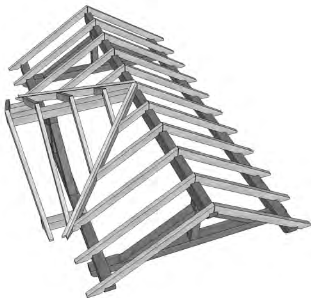
Fig. 7. Roof framing. Common rafters, birdsmouthed at both ends, do not abut at ridge. Dormer ridge is dovetailed to main ridge.
