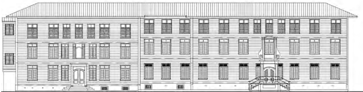
Gravenstraat 16 (left) and Cellier house (right) at 14 after the 1959 removal of the roofs and construction of a continuous third story. The infill section between the two houses dates from the 19th century.
