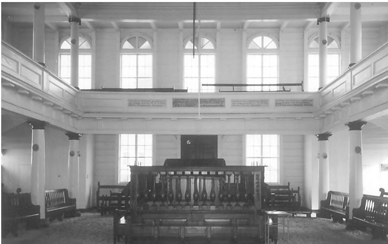
Interior view toward the west façade. To right and left are the stairs toward the women's gallery. The column-to-column distance is 28 ft. 10 in. Side spans are 10 ft. 10 in. The minor dimension of the plan runs left to right in this picture.
