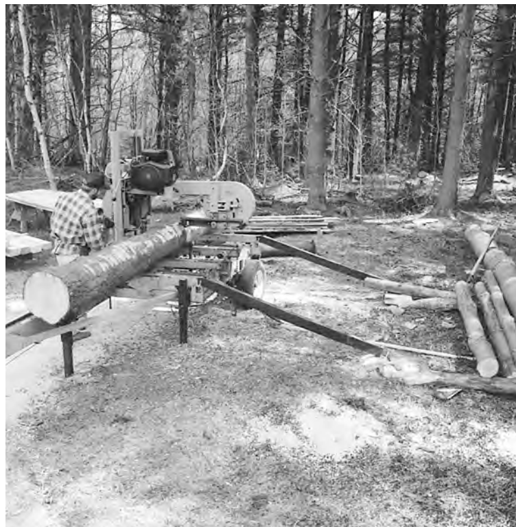
The sawing site should accommodate the logs, the mill and a firewood operation as well as a sawdust pile, slabs and stickered lumber.
