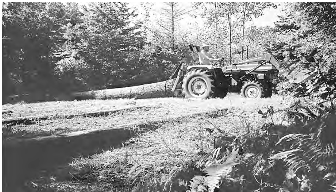
A 30-horsepower 4-wheel drive tractor with logging winch is quite maneuverable off-trail and can pull logs over a ton in weight.
