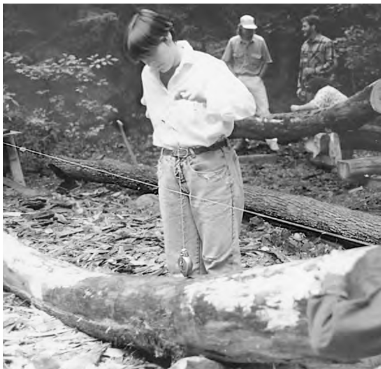
Fig. 14. Plumbing down from the stretched line to get snapping points. For this procedure, the level mark on the log end is plumb.
