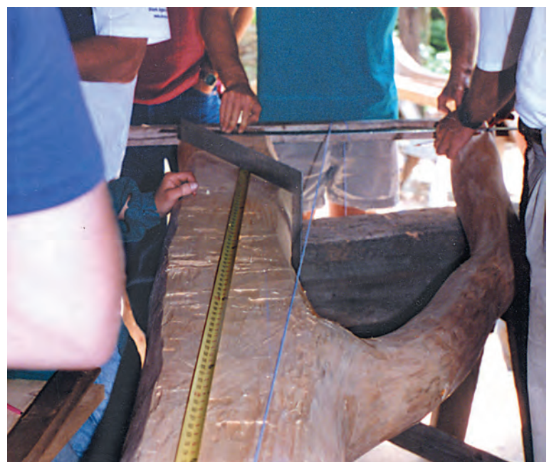
Fig. 11. A forked member requires three ends in plane (one end unseen.)
