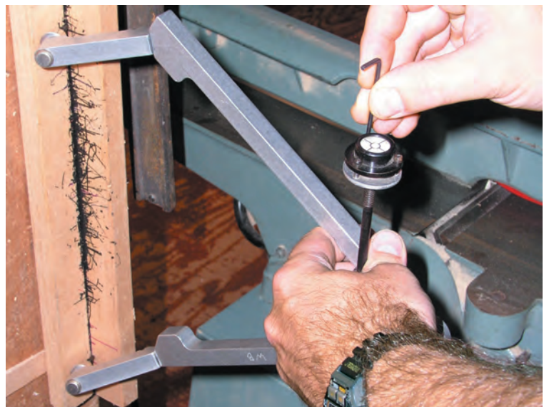
Fig. 4. Calibrating the bubble scribers. The pens must be plumb.
