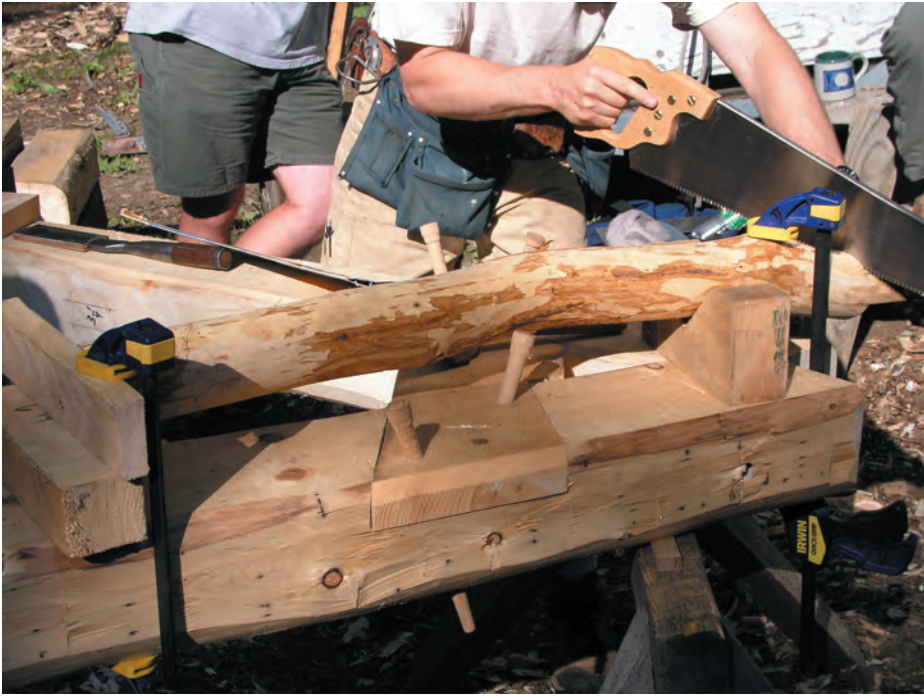
Fig. 2. Logs of whatever size can be kept from rolling by cradling in V-blocks (right end above) or fastening to cleats if small enough (left end), then clamped or dogged in place.
