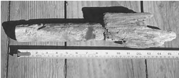
Figs. 10, 11. Original weathered eaves trough support, apparently yellow birch, at the 32x42 Savoy barn, in place at top and salvaged from destroyed barn, above. Shank is 2 in. dia., 9 in. long.
