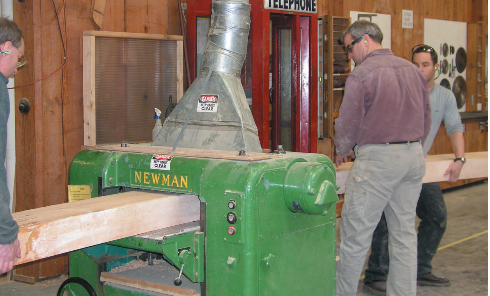
Fig. 8. Damaging effects of excessive noise are well recognized, and efficient hearing protection should be routine. Here, from left, Doug Ward, Duane Beiler (who wears eye protection as well) and Brendan Jones guide a curved glulam through a thickness planer.
