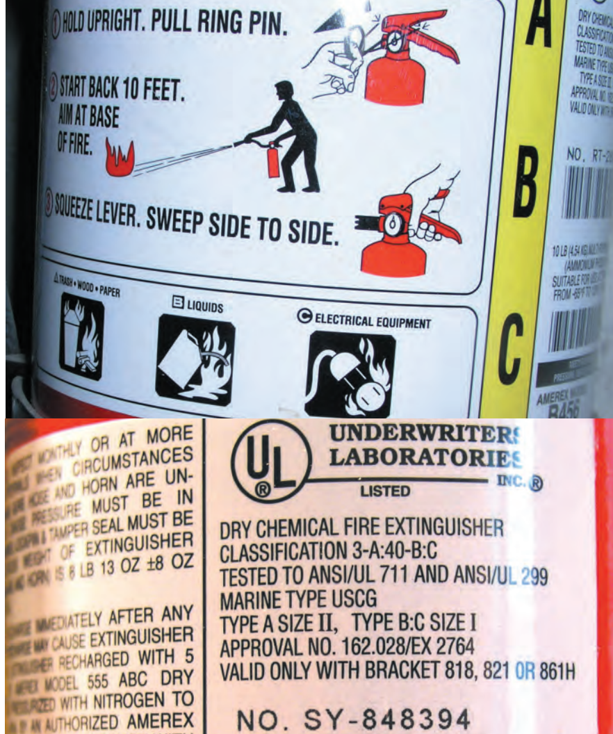
Photos Will Beemer unless otherwise credited Fig. 1. Versatile dry chemical fire extinguisher for woodworking shops. This one will extinguish a wood fire needing three gallons of water or a flammable liquid fire of 40 sq. ft. Electrical fires are not quantified.
