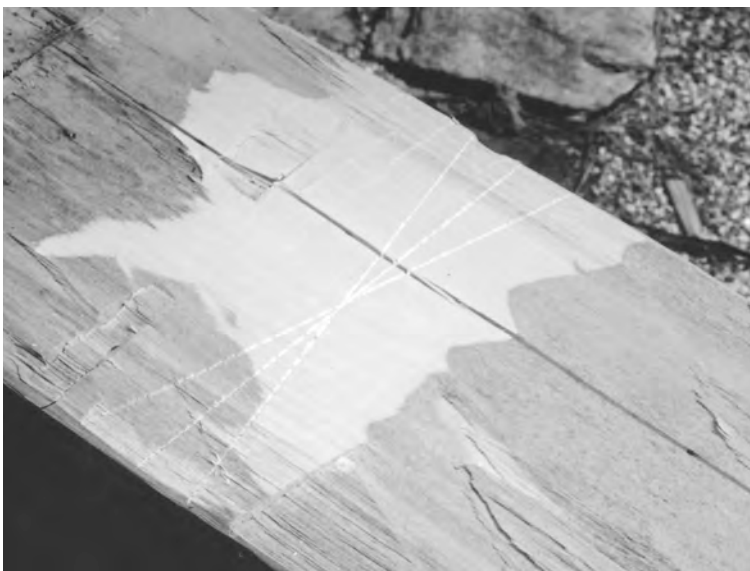
Fig. 4. Level mark on a hewn timber. Freshly planed wood is the paler. This mark graphically represents taking out the winding.
