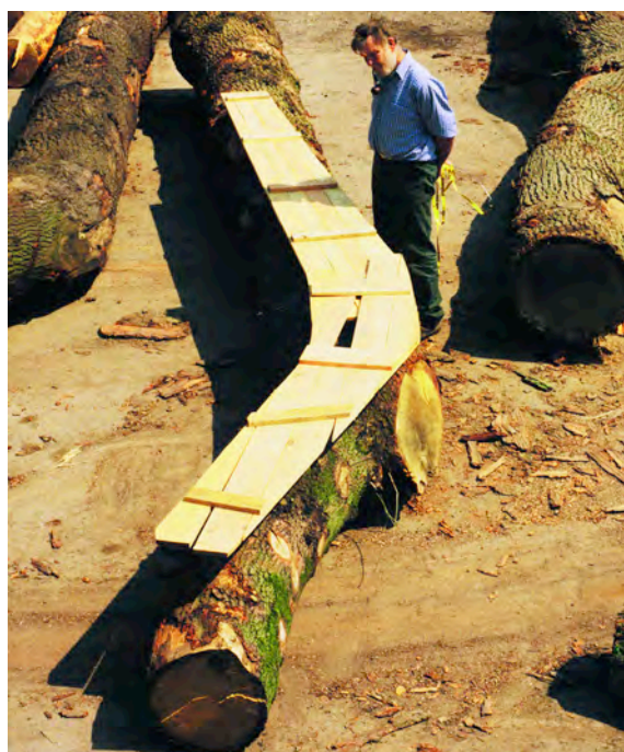
Above, templates were essential to choosing sawlogs for lower crucks. Above right, lower crucks sawn out and under preparation in the workshop.
