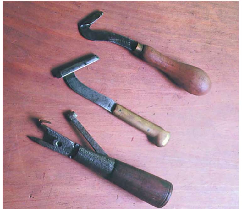
Fig. 15. Race knives. From top, 20th-century fixed-blade style, 19th-century folding model and 18th-century folder with fixed compass point.
