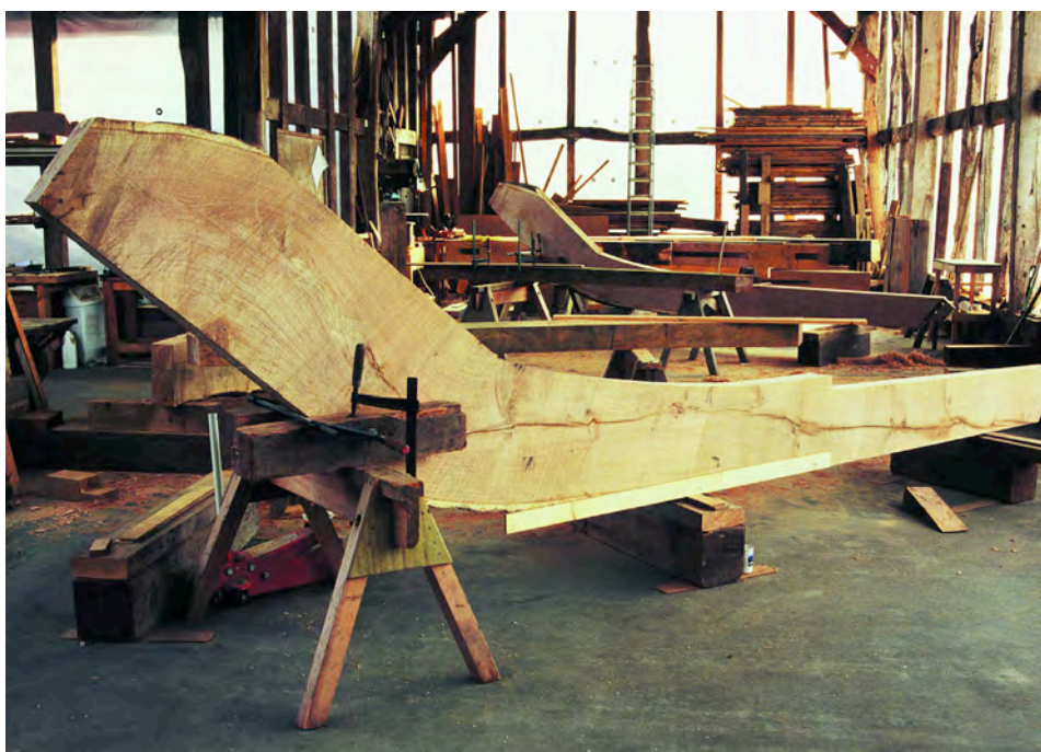
Above, templates were essential to choosing sawlogs for lower crucks. Above right, lower crucks sawn out and under preparation in the workshop.
