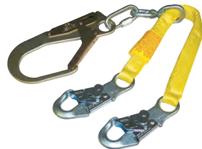
Figs. 6–7. Non-shock-absorbing lanyards to be used only as part of a work positioning system. Lanyards in a fall-arrest system, such as in Fig. 4, must have shock-absorbing capacity.
