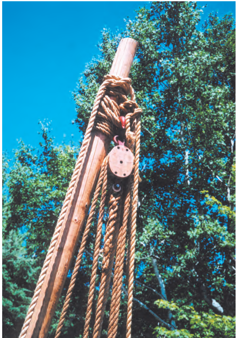
Fig. 7. Choker grip for the load tackle and three guy lines (one fore, two aft) complete rigging at top of gin pole.
