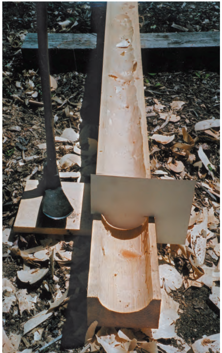
Fig. 14. Gutters are hewn from white pine heartwood with an old gutter adze. A simple template is used to maintain a consistent profile in the 4x6 workpiece.
