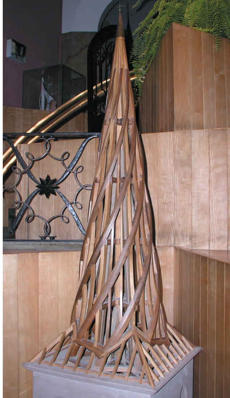
Fig. 10. Masterpiece twisted steeple frame model at Strasbourg.
