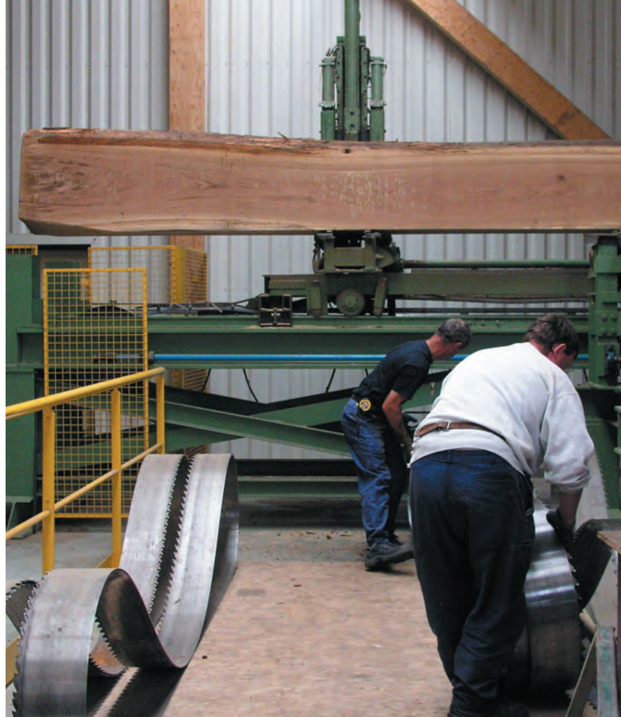
Fig. 5. Perrault sawyers prepare large bandsaw blades in immaculate sawmill. Log on carriage will yield a timber about 30 in. square. Figs. 6–8. Below, below left and above left, sophisticated 18th-century timber work from the north tower of the Église Saint-Sulpice in Paris, under repair at Ateliers Perrault near Angers.
