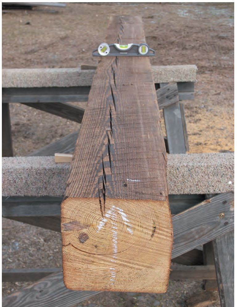
Fig. 5. Wedging the timber to level at “zero” point along surface.
