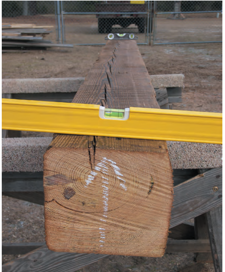
Fig. 4. Determining the amount of wind by comparing levels.
