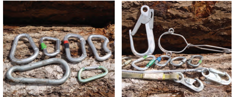
Figs. 7–8. At left, nonlocking snaphooks not acceptable to OSHA. Right, acceptable snaphooks, which must also be compatible with equipment they are attached to. OSHA considers a hook compatible when the diameter of the D-ring it's attached to is greater than the longest inside length of the snaphook.
