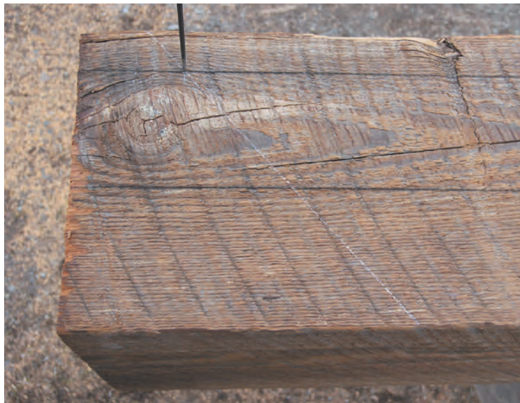
Fig. 10. Awl points out intersection of shoulder and reference lines.
