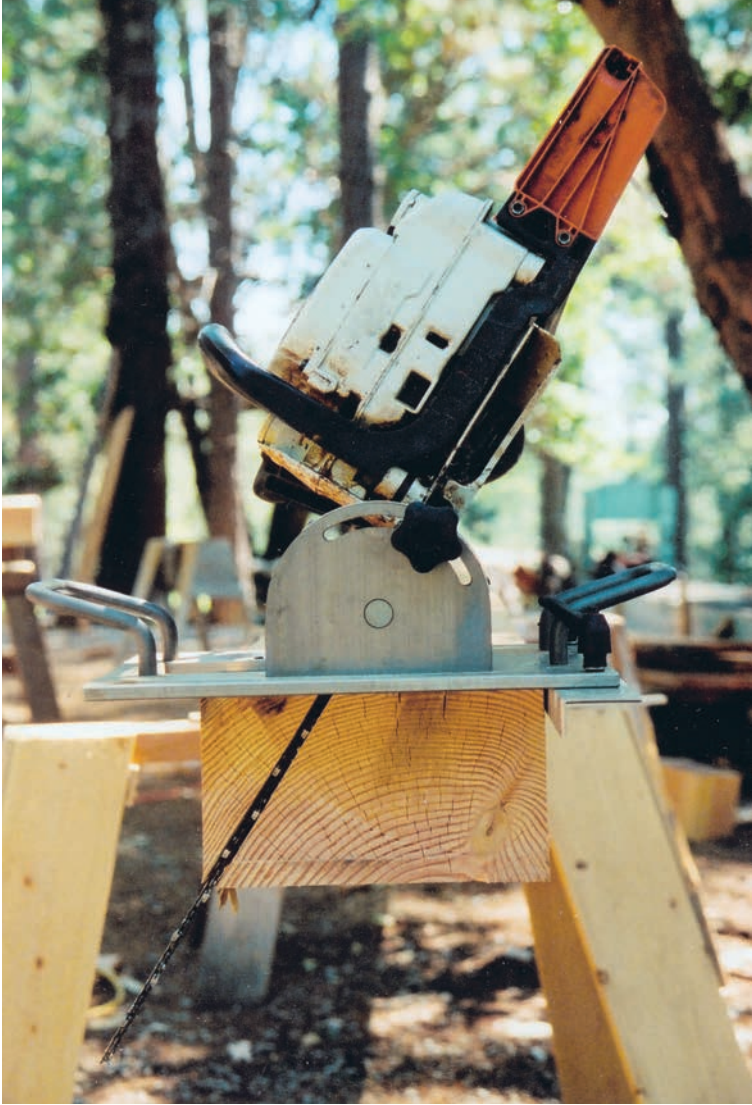
Fig. 4. Accutech base adjusted for bevel cut at fixed distance from timber edge. Chain is filed for ripping.
