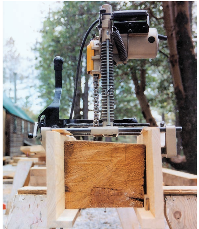
Fig. 7. Chain mortiser mounted on jig ready to cut mortise perpendicular to reference surface.
