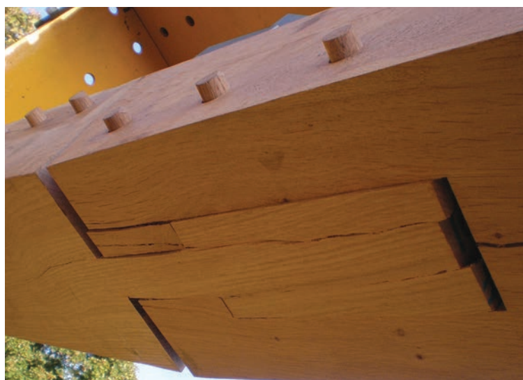
Gooseneck pegged scarf, failure in shear parallel to grain.
