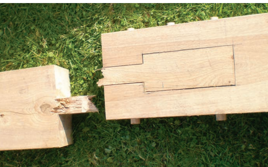
Gooseneck pegged scarf, failure in tension parallel to grain.
