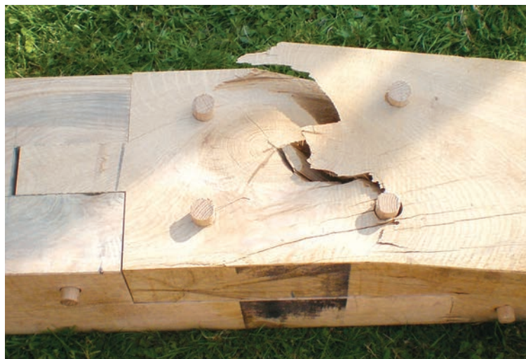
Bridled, face-halved and pegged scarf tested to destruction. Short grain at large knot made contest unfair, left joinery untested.
