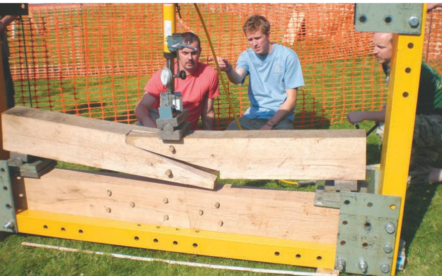
Hydraulic ram device, designed at the University of Bath, UK, testing and destroying edge-halved, splayed and pegged oak scarf joint.
