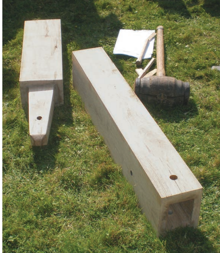
Post scarf with tapered mortise and tenon and double-axis pegging, normally used for in situ repair. In bending it failed at mortise walls.
