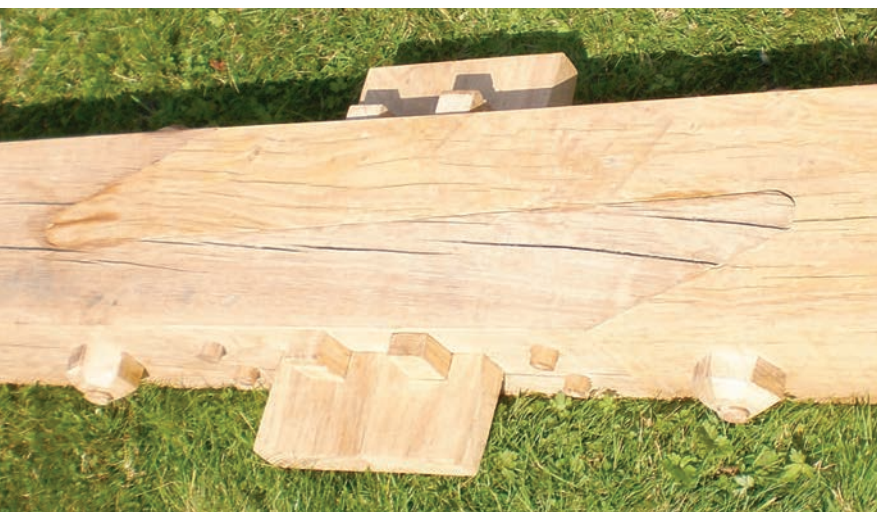
Very rare machine-cut, undersquinted, radiused, edge-halved, outside-wedge-keyed, wooden-bolted and pegged oak scarf joint before testing.
