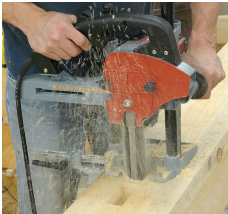
Fig. 7. Cross-grain mortiser (here the Mafell) has fixed width of cut, adjustable distance from edge and no limit on mortise length.
