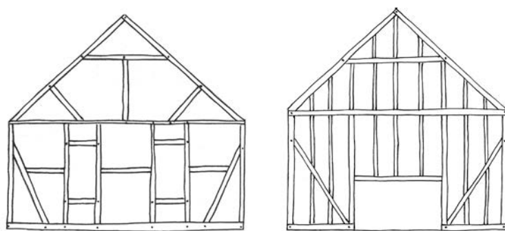
St. Kitts Anglican Church rectory endframe at left compared with ca.-1765 Clermont house frame in Berryville, Virginia.
