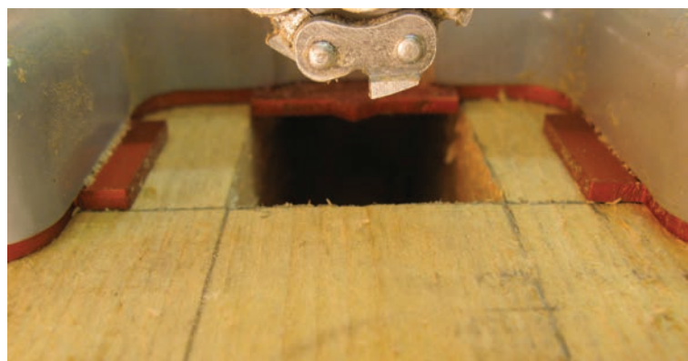
Fig. 3. SwissPro's registration plate aligns at mortise ends and width.
