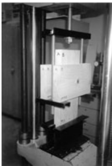
Figure 2. — Riehle test machine setup.
